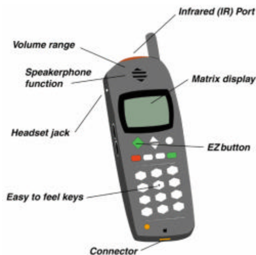
Figure 8.1.1 – Cellular Phone Reference Design
