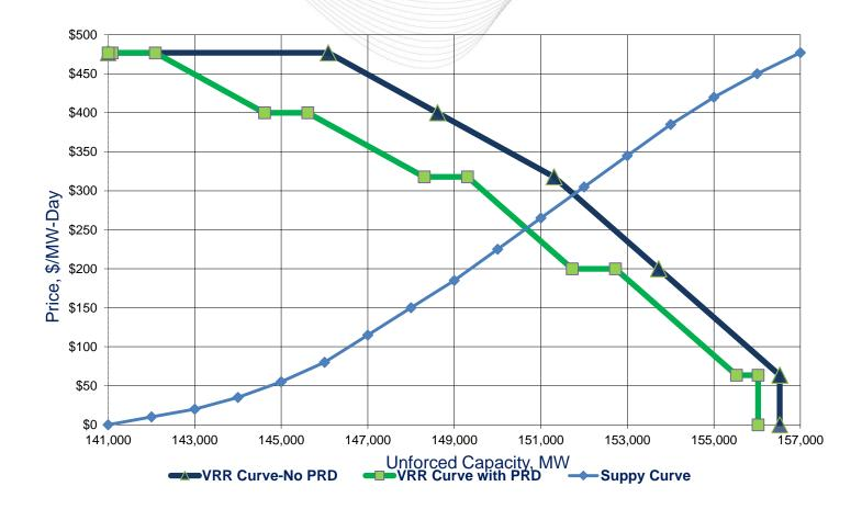
PRD will shift or change the demand curve which will reduce the overall capacity requirement
