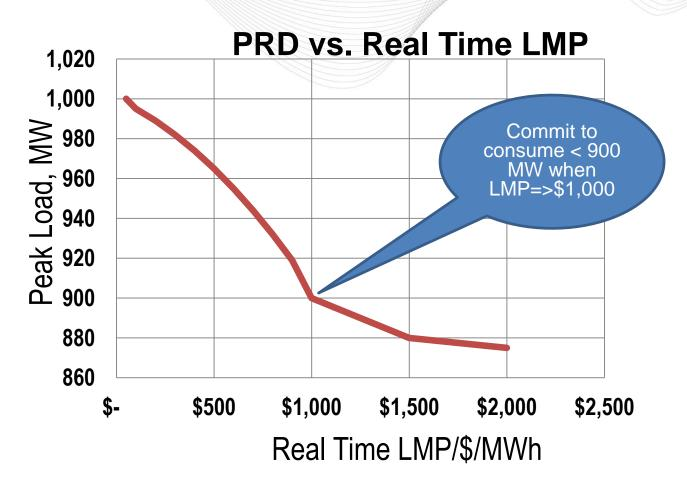
Price Responsive Demand (PRD) – load that will automatically respond to energy prices and be off the grid during PJM emergency in exchange for reduction in capacity requirement.
